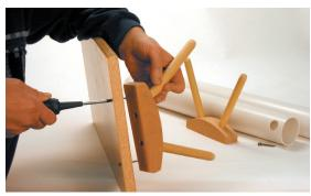
Insert screws through holes in bottom of base plate (with screw heads in countersinks). Line up holes in bottom of doweled bracket with screws and tighten screws securely into doweled bracket with Phillips head screwdriver as shown in photo.
